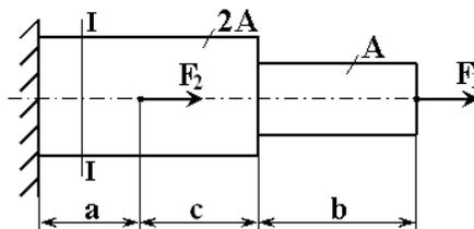
$$F_2 = 20 \text{ кН}; F_1 = 10 \text{ кН}; A = 100 \text{ мм}^2; a=b=c=1 \text{ м}; [\sigma]_p = 100 \text{ МПа}.$$
