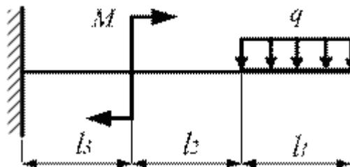
$$l_1 = l_2 = l_3 = 1 \text{ м}; M = 10 \text{ кН}\cdot\text{м}; q = 5 \text{ кН/м}$$
